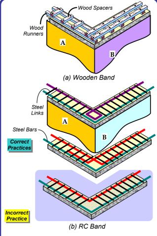
Figure 4: Horizontal Bands in masonry buildings - RC bands are the best.
