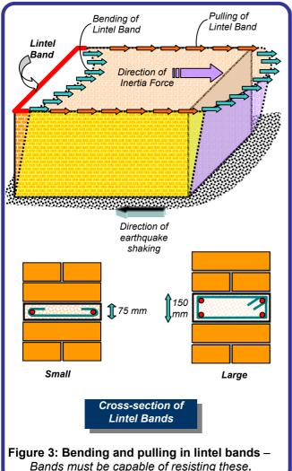
Bands must be capable of resisting these.
